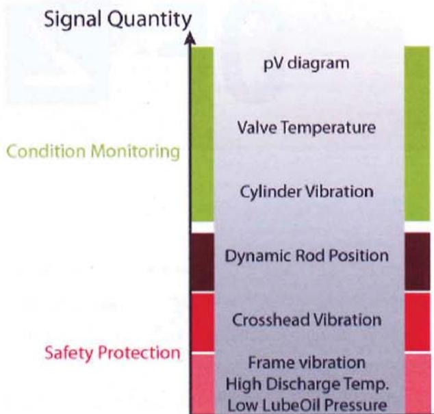
**Figure 4.** Typical levels of safety protection and condition monitoring for reciprocating compressors.
