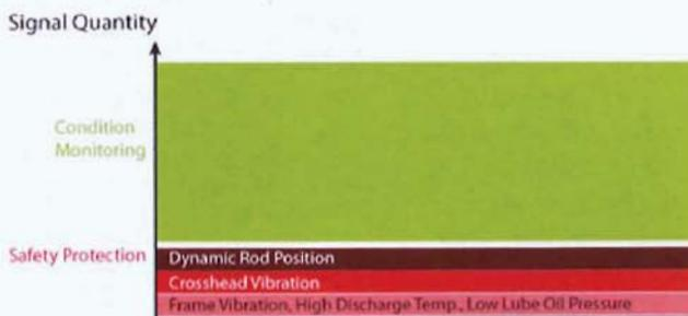
**Figure 3.** Typical methods of safety protection for reciprocating compressors.
